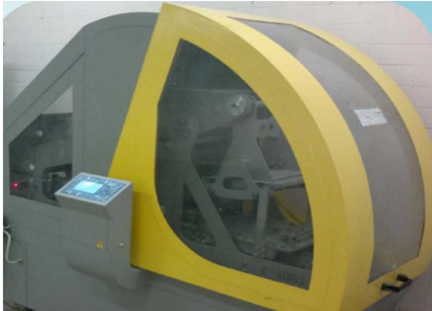
Fig. 2. The Roller Compactor
